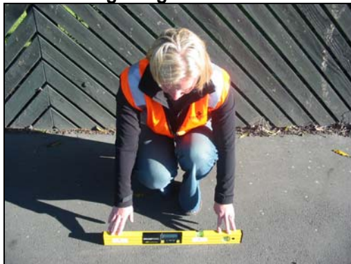
Figure PL37.1 Measuring Longitudinal Gradient
