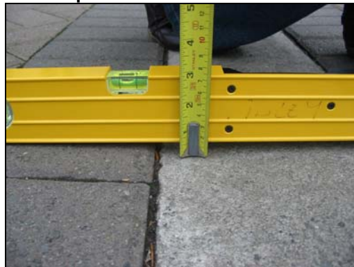
Figure PL38.2 Example of How to Measure Stumbling Hazards
