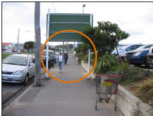
The obstacle is located on both the kerb and rear of the footpath and is counted as one obstacle
