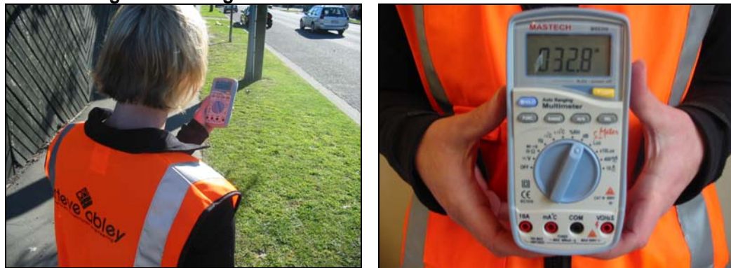
Figure PL20.1 Measuring Noise Using a Multimeter
