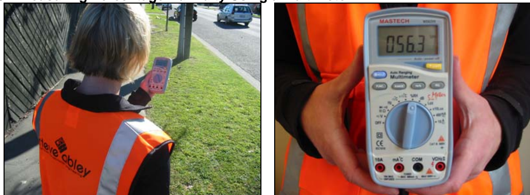
Figure PL18.1 Measuring Percentage Humidity Using a Multimeter
