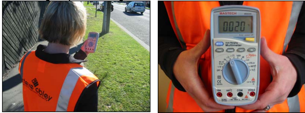
Figure PL19.1 Measuring Temperature Using a Multimeter
